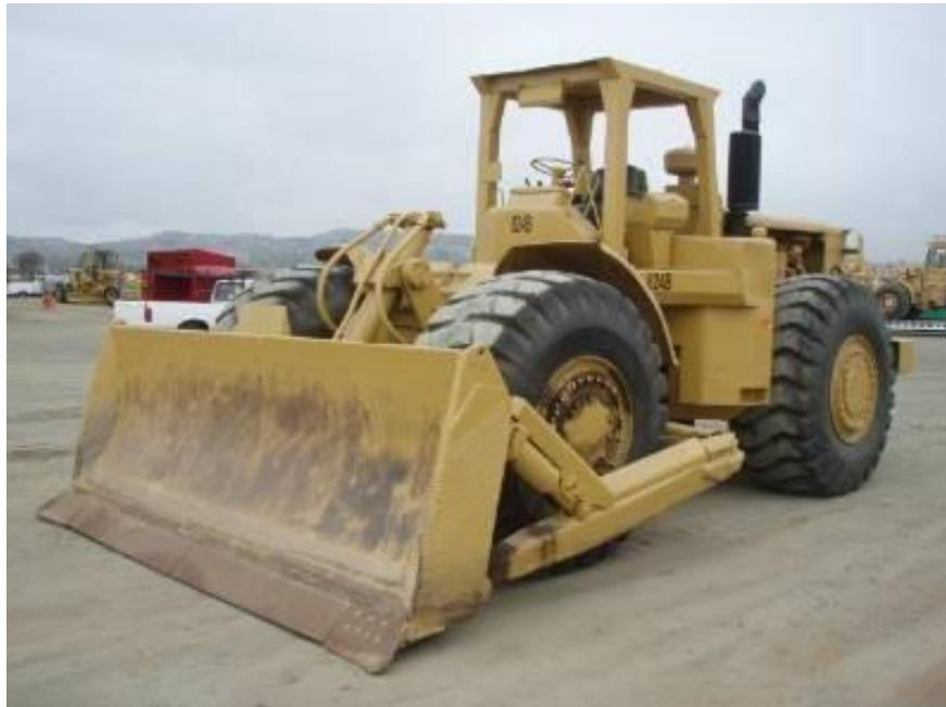
**Figura 1. Tractor bulldozer a rueda**
